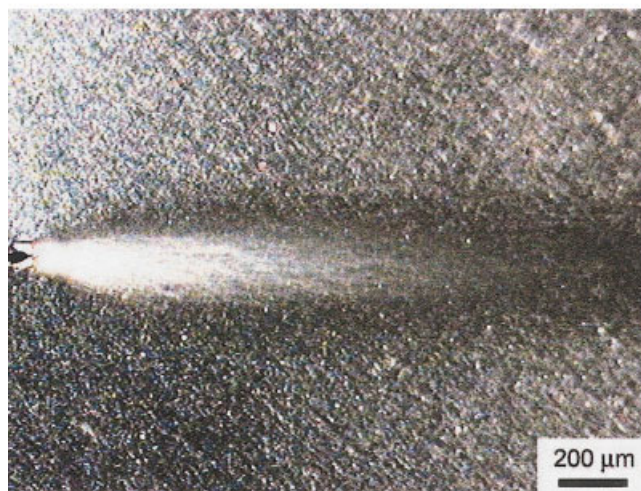
Figure 3 TOM of DN-4PB Charpy impact damage zone of PP/CaCO 3 nanocomposite: (a) bright field and (b) cross polarized field. The crack propagates from left to right. [Color figure can be viewed in the online issue, which is available at www.interscience.wiley.com .]
